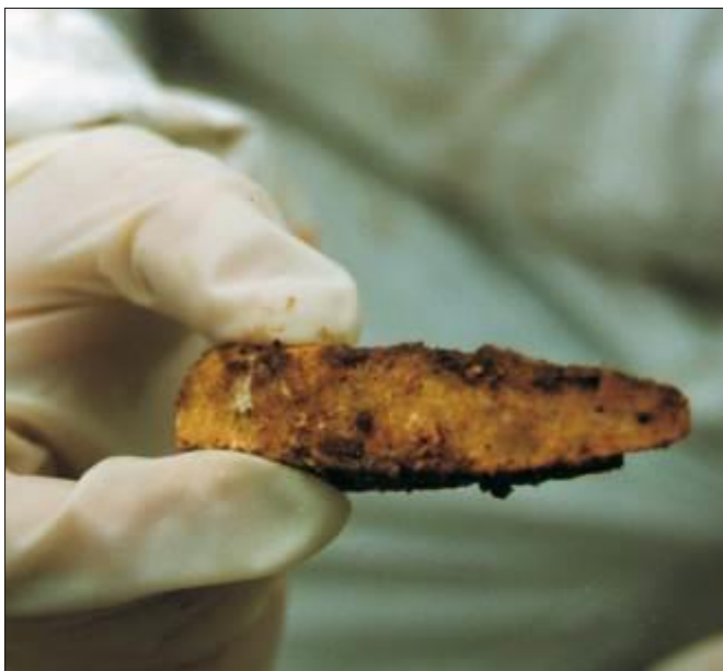
Fig. 2: Fragment of crystalline TNT
